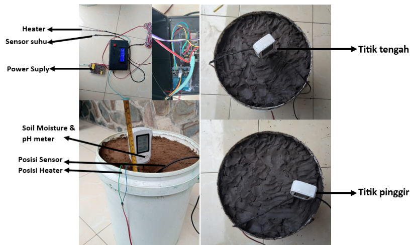
Figure 5. Prototype of Conductivity Measurement System
