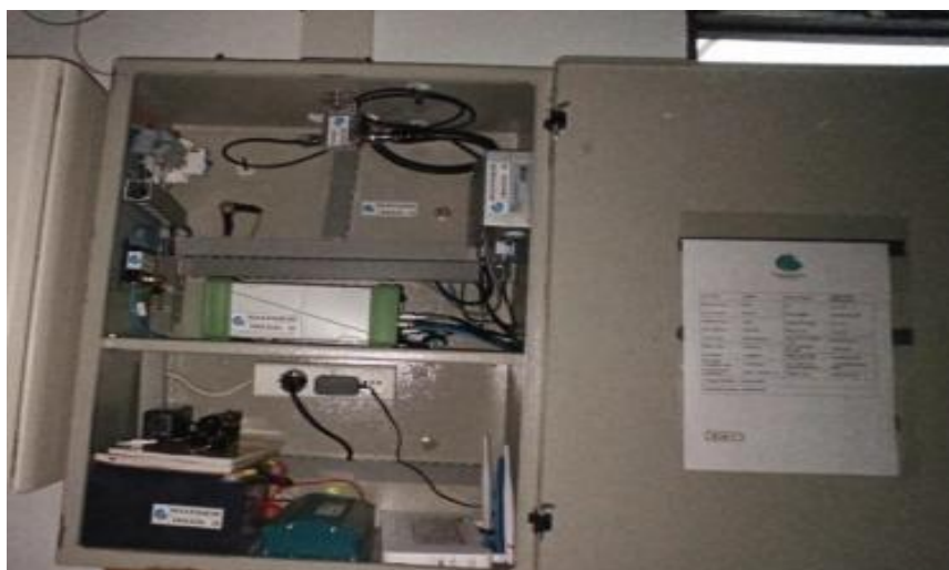
Figure 11. Receiver and Indoor Equipment of CORS CSAM Station
